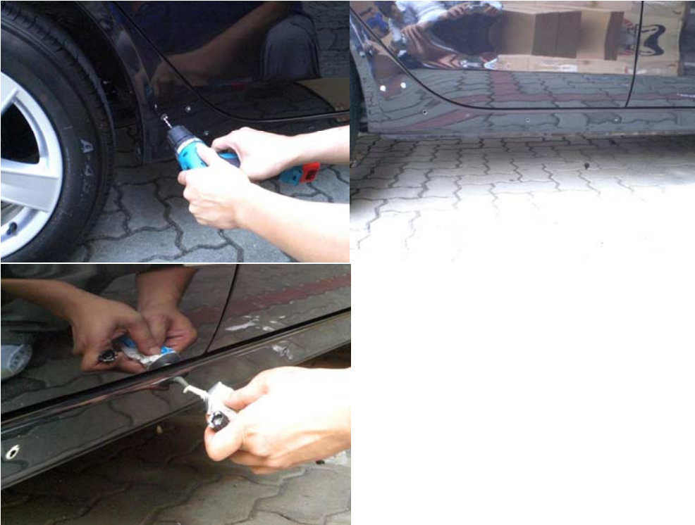
Picture 29/30/31: Use a 3mm drill bits to drill pilot holes at the middle of the marker, than enlarge the pilot holes by using 7.5mm drill bits. Then apply silicon to the holes as picture shown.
